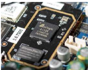
Amlogic A113X 64-bit quad-core Arm Cortex-A53 processor for high resolution wireless streaming
