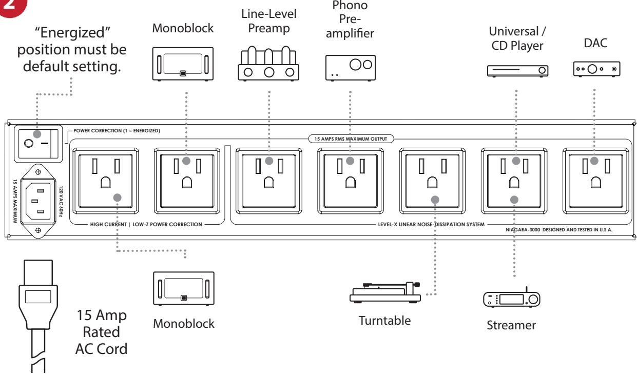
**Note:** Banks 3 through 7 are subject to many variables and circuit conditions, so experimentation for best results is encouraged. Power amplifiers **must** be connected to banks 1 or 2.
